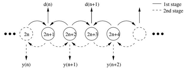
**Fig. 3.** Two-step implementation of wavelet transform using lifting.
