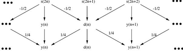
Fig. 4. Lifting Architecture for 5/3 wavelet
