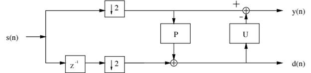
**Fig. 2.** Lifting implementation of wavelet transform.  $P$  corresponds to the prediction stage, and  $U$  to the update stage.
