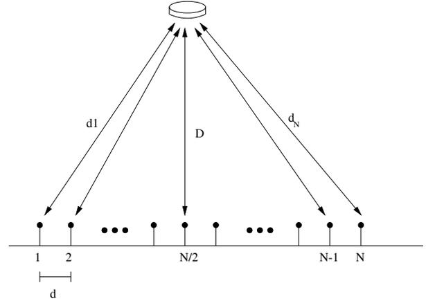
Fig. 5. Placement of sensors and central node
