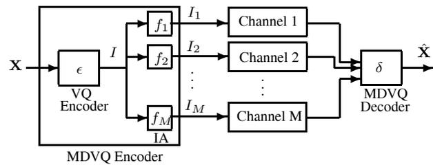
Fig. 1. A communication system based on MDVQ.
