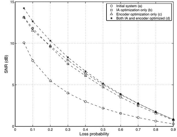
**Fig. 3.** Performance of MDVQ for Gauss-Markov source ( $M = 2$ ,  $k = 2$ ,  $R_1 = R_2 = 2$  bits/sample).
