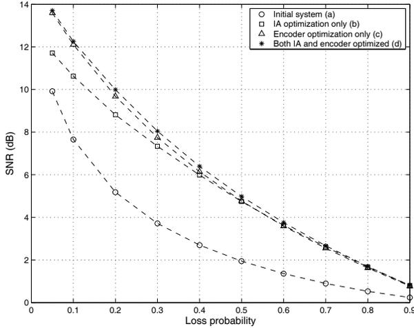
**Fig. 2.** Performance of MDVQ for iid Gaussian source ( $M = 2$ ,  $k = 2$ ,  $R_1 = R_2 = 2$  bits/sample).
