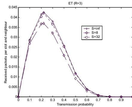
Figure 5. Effective throughput in a network of 1000 nodes, for different values of  $\alpha$ , when t-MPR collisions are considered. Plots show the cases of 8, 32 and infinite number of available TS.
