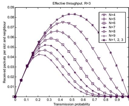
Figure 3. Effective throughput for different number of neighbouring nodes and a contention period of length 3.
