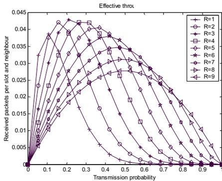
Figure 2. ET for different values of the transmission probability ( $\alpha$ ) and contention period ( $R$ ) length for nodes with 9 neighbours
