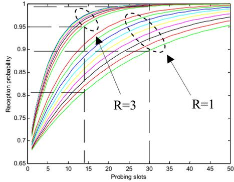
Figure 4. Reception probability vs. number of probing slots for optimum values of  $\alpha$ . For two values of  $R$ , different number of neighbours are chosen (1 for upper curves, 9 for lower curves).
