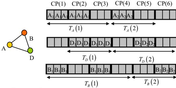
Figure 1. Transmission pattern within the probing channel
