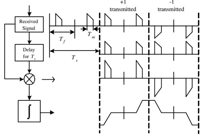
Fig. 1. Differential receiver ( $N_f = 2$ )
