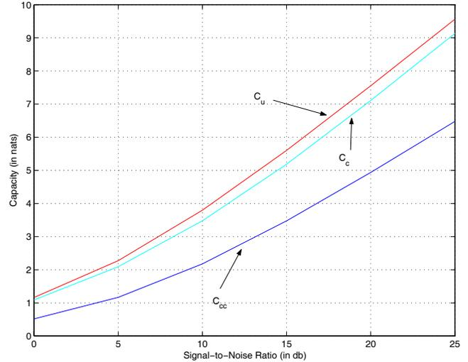
**Fig. 2.** Capacity vs SNR for  $n_t = 2$  and  $n_r = 2$ , i.e.,  $2 \times 2$  Rayleigh channel matrix. Note that  $C_u$ ,  $C_c$  and  $C_{cc}$  denote the capacity of uncorrelated, correlated at the receiver end and correlated at both transmitter and receiver ends, respectively.
