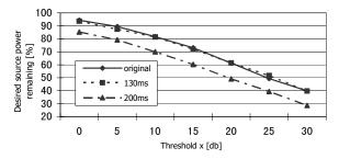
Fig. 2: Approximate WDO against the threshold x for a DFT size of 512 and a male-male-female combination.
