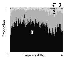
Fig. 1: Histogram of the number of active sources: 0, 1, 2 or 3 for a male-male-female combination recorded with a reverberation of 200 ms and for a DFT size of 512.
