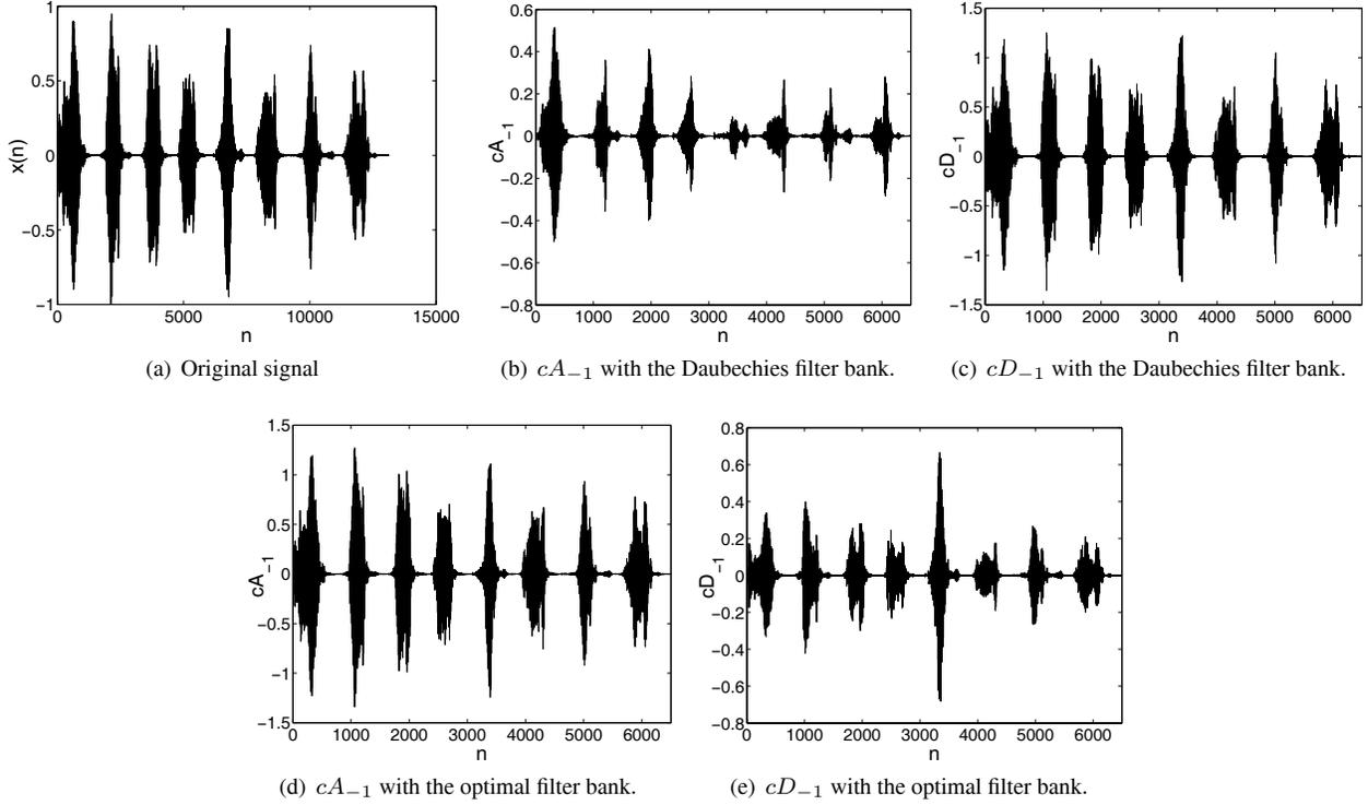
Fig. 2. Decomposition of a signal  $x(n)$  using the Daubechies wavelets and the optimized wavelets.
