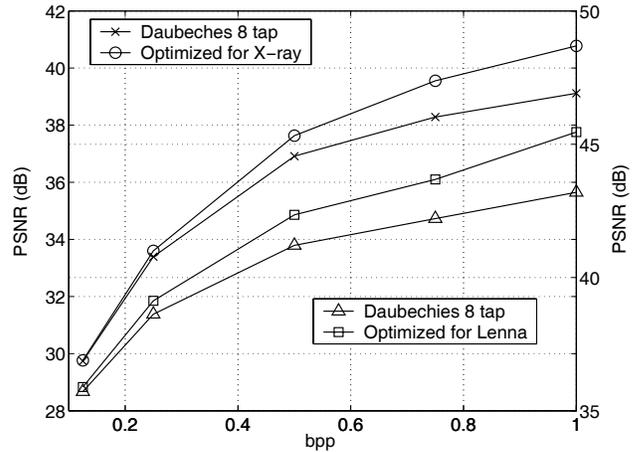
Fig. 3. PSNR vs bpp for the Lenna (bottom) and X-ray (top) test images, coded with the optimized filters as well as the original Daubechies 8 tap filters. The top two graphs follow the right hand side y-axis while the bottom two follow the left y-axis.
