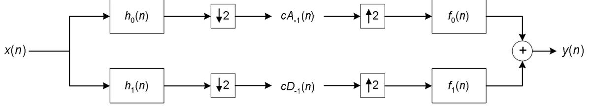
**Fig. 1.** Implementation of a single stage wavelet transform using a filter bank.
