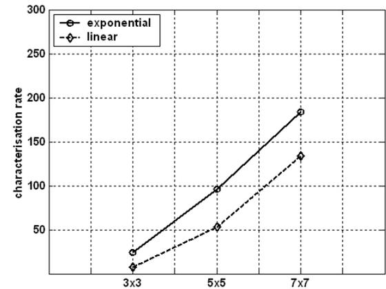
Figure 3: Characterization rate of the 2-D exponential filter and the 2-D linear filter with respect to the filter orders.
