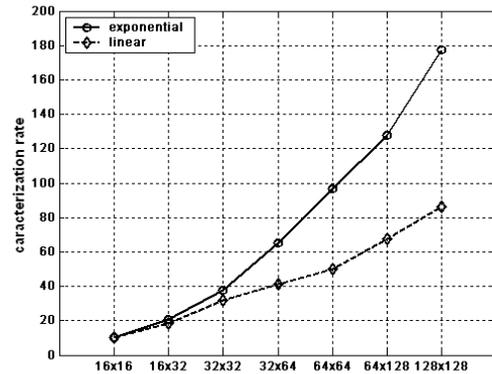
**Figure 5:** Characterization rate of the 2-D exponential filter and the 2-D linear filter versus the texture image size
