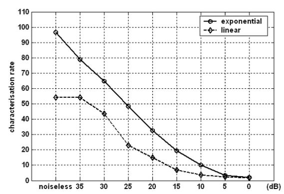
Figure 4: Characterization rate of the 2-D exponential filter and the 2-D linear filter for various SNR values.
