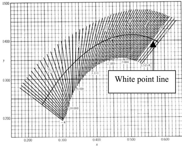
Figure 1. Isotherm lines and white point line in (x, y)-chromaticity diagram.
