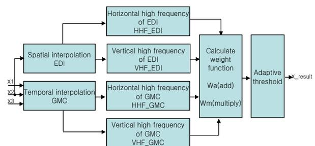
Fig. 1. The block diagram of the proposed algorithm.
