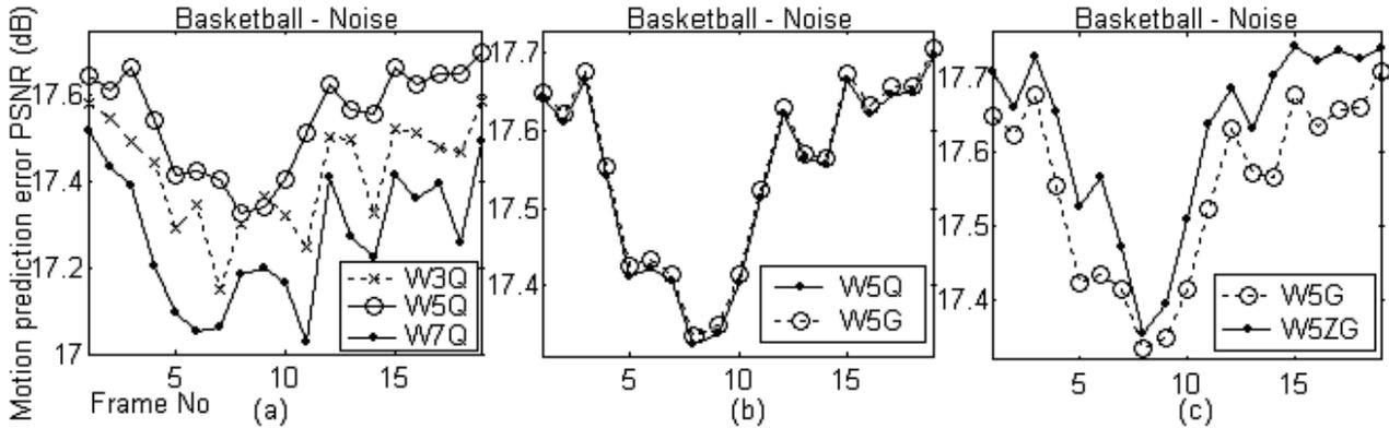
Fig. 2. (a) 1st (W3Q), 2nd (W5Q) and 3rd (W7Q) order filtering using Quadratic fitting (b) Gaussian (W5G) and Quadratic (W5Q) fitting for the 2<sup>nd</sup> order Gradient filter (c) With (W5ZG) and without (W5G) zero-padding using the 2<sup>nd</sup> order Gradient filter.
