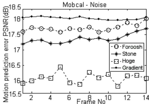
Fig. 3. PSNR versus frame number for local (block-based) motion compensated prediction with Gaussian noise
