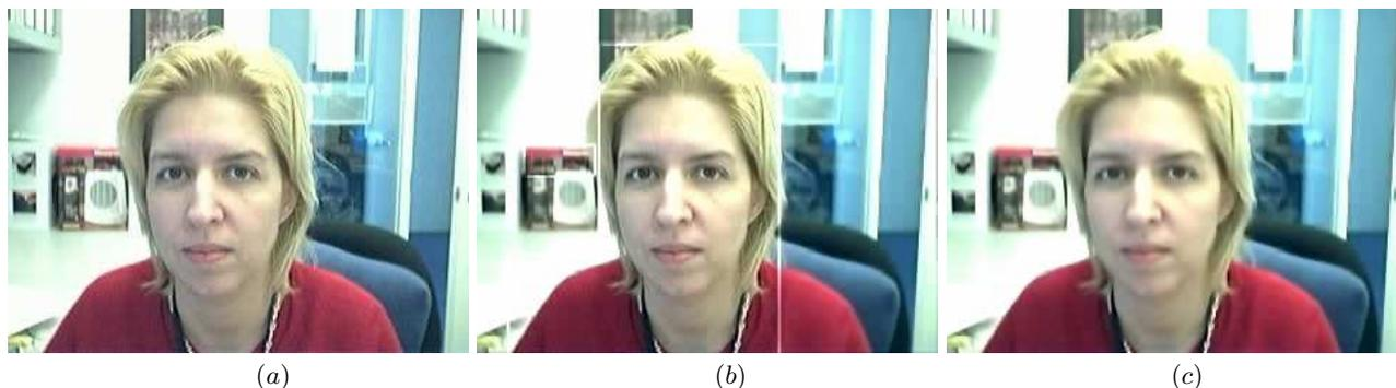
**Fig. 3.** (a) Original frame acquired using a Logitech Notebook Pro camera, (b) frame that has been filtered using our proposed method and then coded at 150 kbps/s using a H.263 video codec, and (c) frame that has been filtered using *equal* anisotropic diffusion and then coded at 150 kbps/s using a H.263 video codec.
