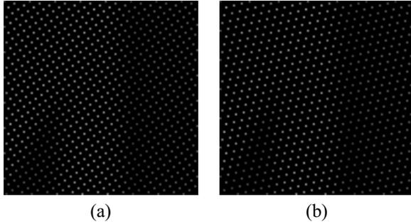
**Fig. 4.** A  $100 \times 100$  pixel region in the upper left corner of the image showing subsampling patterns: (a) rectangular; (b) approximately hexagonal. From a distance of about 8 - 10 times the height of the figure, the reader should be able to see that the density of samples in (b) is lower than in (a).
