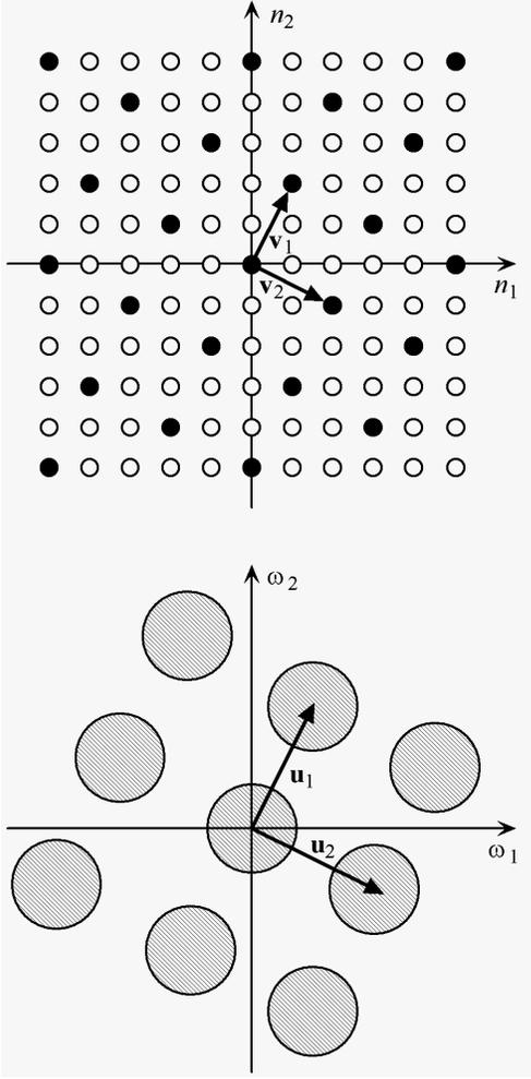
**Fig. 1.** An illustration of 2-dimensional subsampling in the space domain (top) and the frequency domain (bottom).
