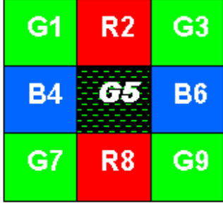
Figure 3. A typical RGB color filter array with pixel-centered interpolation
