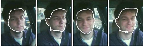
**Fig. 3.** Contour tracking applied to driver's face extraction, using the weighted gradient (skin chroma being the feature of interest). Randomly chosen images from a video sequence.
