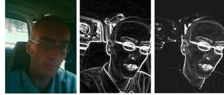
**Fig. 2.** (a) Original image, (b) usual euclidean gradient on Lab, (c) featured weighted gradient, the feature being the skin chroma.
