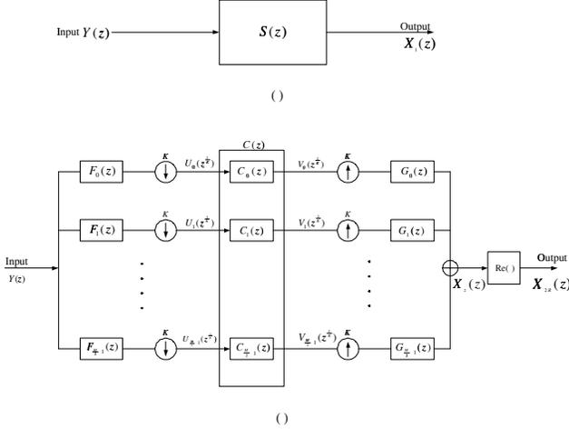
**Fig. 1.** (a) An arbitrary LTI system  $S(z)$ . (b) A subband approximation of the system  $S(z)$ .
