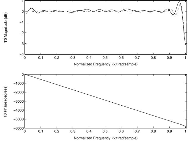
Fig. 2. Magnitude and phase of the distortion function
