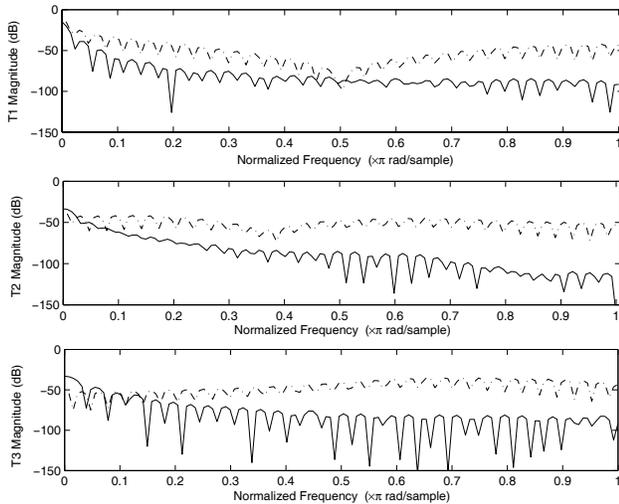
Fig. 4. Magnitude of the aliasing functions
