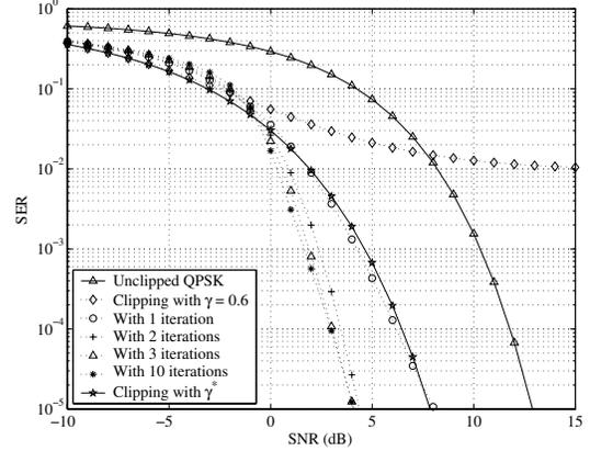
**Fig. 6.** SER for unclipped OFDM; clipped OFDM with  $\gamma = 0.6$  for iterations 0, 1, 2, and 10; and clipped OFDM with  $\gamma = \gamma^*$ .
