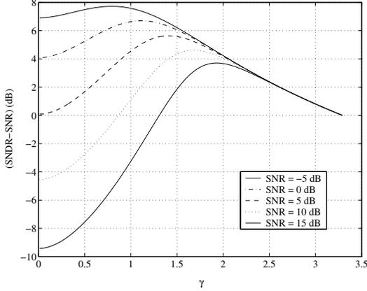
Fig. 3. Gain in SNDR as a function of  $\gamma$  for various SNRs.
