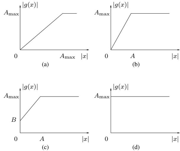
**Fig. 1.** Some nonlinear mappings under the peak amplitude constraint: (a) Soft limiter; (b) soft limiter with gain  $A_{\max}/A \geq 1$ ; (c) limiter with amplitude translation and scaling; (d) hard limiter.
