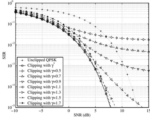
**Fig. 5.** SER vs. SNR curves for unclipped OFDM, clipped OFDM with  $\gamma = 0.5, 0.7, \dots, 1.7$ , and clipped OFDM with  $\gamma = \gamma^*$ .
