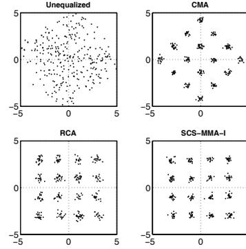
**Fig. 4.** Signal constellation of 16-QAM (a) Unequalized, (b) CMA, (c) RCA, and (d) SCS-MMA-I. The step-sizes are  $8.0 \times 10^{-4}$ ,  $4.0 \times 10^{-4}$  and  $5.0 \times 10^{-5}$  for RCA, SCS-MMA-I and CMA, respectively.
