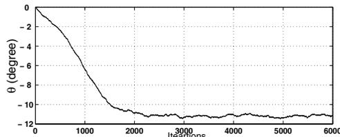
**Fig. 3.** Rotator phase estimation in CMA.
