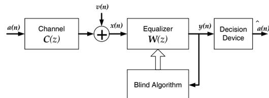
Fig. 1. Blind equalization in the baseband.
