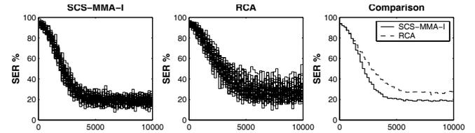
**Fig. 6.** Ensemble average SER for 64-QAM, SNR = 20dB.  $\mu = 8.0 \times 10^{-5}$  for RCA and  $\mu = 2.0 \times 10^{-5}$  for SCS-MMA-I. SCS-MMA-I is not only less dispersive but its steady-state SER is less than that of RCA by 10 units.
