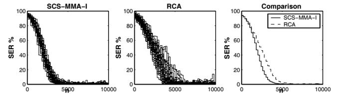
**Fig. 7.** Ensemble average SER for 64-QAM, SNR=30dB. All parameters are same as those in Fig. 6.
