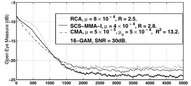
**Fig. 5.** Ensemble average ISI for 16-QAM.  $\mu = 8.0 \times 10^{-4}$  for RCA,  $\mu = 4.0 \times 10^{-4}$  for SCS-MMA-I and  $\mu = 5.0 \times 10^{-5}$  for CMA.
