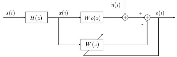
**Fig. 1.** Block diagram of the adaptive system modelling simulation.
