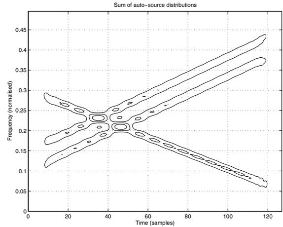
**Fig. 1.** Sum of the auto-source TFDs of the three chirp source signals.
