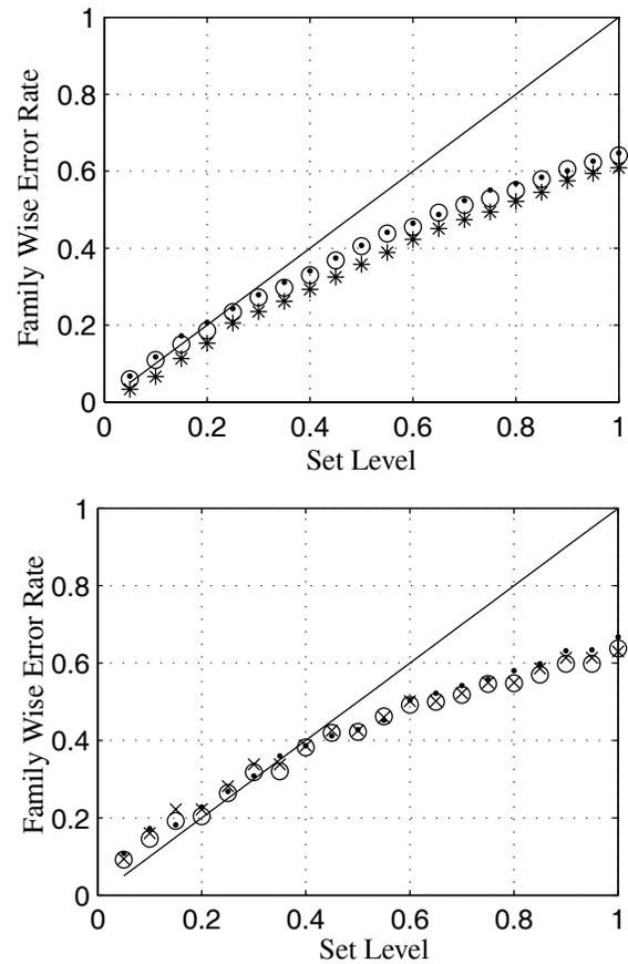
**Fig. 3.** FWE for (top) normal approximation and (bottom) bootstrap based detector. SNR = -3 dB (\*), SNR = -6 dB ( $\circ$ ), SNR = -9 dB ( $\bullet$ ).
