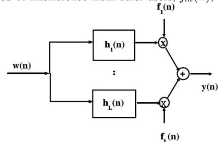
Fig. 1. Transmission channel with multi-path and Doppler effects
