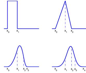
Fig. 1. Nonuniform B-splines of degree 0 to 3.
