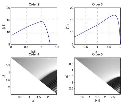
**Fig. 5.** Performance of symmetric B-splines of degree 2 (top-left) to 5 (bottom-right) as function of the knot placement, when interpolating a bandlimited signal with constant spectrum.
