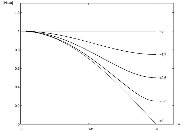
Fig. 3.  $|H_l(\omega)|$ -s of linear interpolation ( $L = 8$ )
