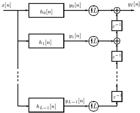
Fig. 2. The interpolation part using polyphase filters
