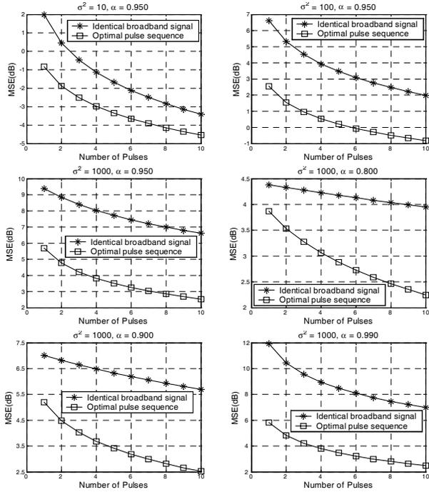
Figure 2: MSE reduction for different values of  $\alpha$  and  $\sigma^2$ .
