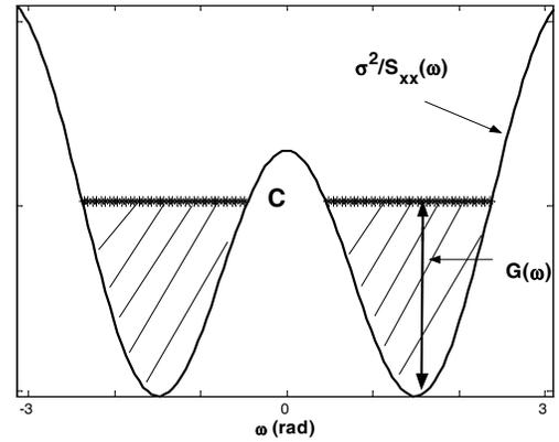
Figure 1: Water-filling distribution of spectral energy
