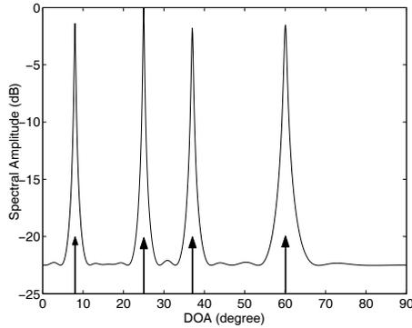
**Fig. 5.** MUSIC spatial spectrum for four signals with equal power (SNR = 0 dB) at directions 8°, 25°, 37°, and 60° by a two-level decomposition.
