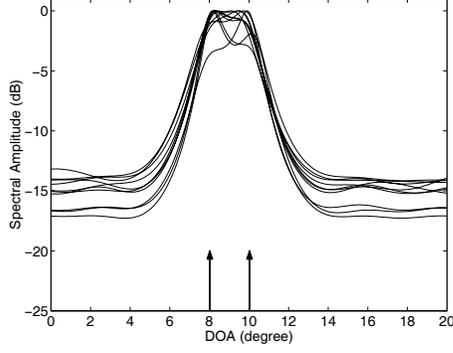
**Fig. 1.** MUSIC spatial spectrum for two signals with equal power (SNR = -5 dB) from  $8^\circ$  and  $10^\circ$  by ten batches.
