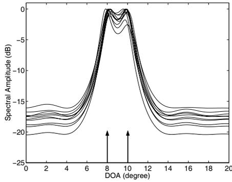
**Fig. 2.** WP-MUSIC spatial spectrum for two signals with equal power (SNR = -5 dB) from  $8^\circ$  and  $10^\circ$  by ten batches.
