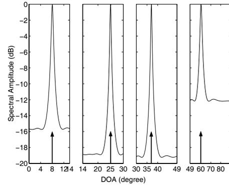
**Fig. 6.** WP-MUSIC spatial spectrum for four signals with equal power (SNR = 0 dB) at directions 8°, 25°, 37°, and 60° by a two-level decomposition.
