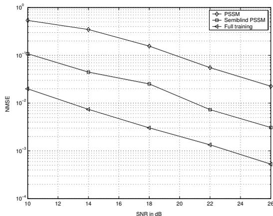
Fig. 3. retransmission channel estimation performance over random channels
