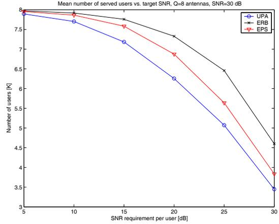
**Fig. 2.** Number of served users as a function of the SNR requirements for the admission control mechanisms.
