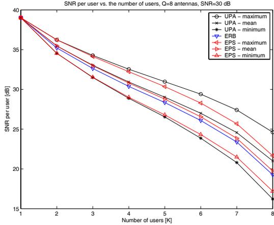
**Fig. 1.** Maximum, mean, and minimum output SNR as a function of the number of users for the scheduling mechanisms. For the ERB, the maximum, mean, and minimum coincide.
