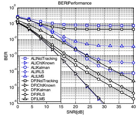
Fig. 3. BER improvement with channel tracking for the decision feedback detection scheme (AL and DF denote the Alamouti-based and our decision feedback detection scheme).
