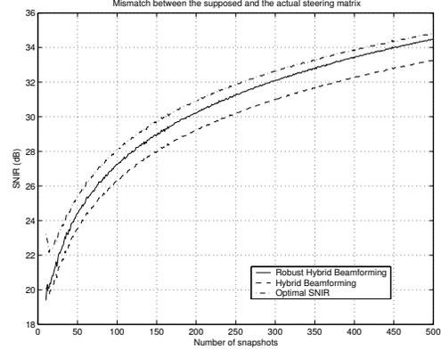
Fig. 2. Output SNIR with a steering mismatch of  $5^\circ$
