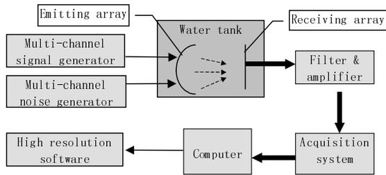
**Figure 5 The structure of multi-reflector multi-dimensional joint estimation experiment system**
