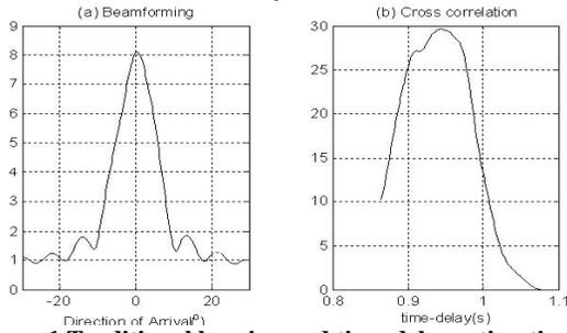
Figure 1 Traditional bearing and time-delay estimation
