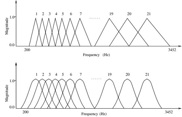
**Fig. 2.** Illustration of the explicit filter bank used in conventional MFCC feature computation (shown on top of figure) and the implicit filter bank argued in WOSA-MFCC feature computation (shown in the bottom of figure).
