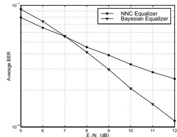
Fig. 5. The performances of nearest neighbor classifier (NNC) equalizer and our Bayesian equalizer for satellite channel with 2 paths and Rician factor  $K = 9\text{dB}$  and  $f_d = 10\text{Hz}$ .
