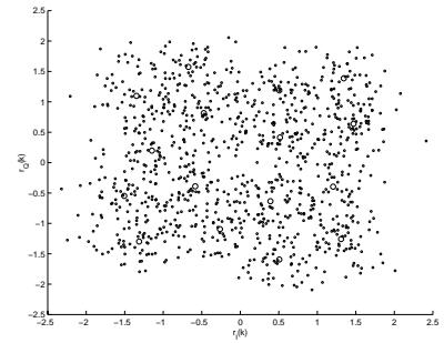
Fig. 3. The centers of 16 channel states (denoted by circles) obtained via FCM clustering when  $E_b/N_0 = 7\text{dB}$ ,  $K = 12\text{dB}$ , and  $f_d = 20\text{Hz}$ .
