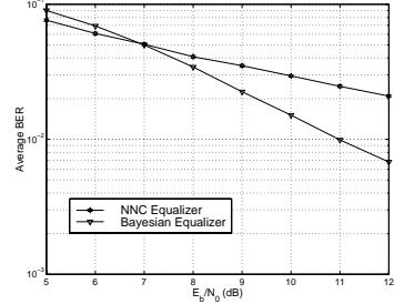
Fig. 4. The performances of nearest neighbor classifier (NNC) equalizer and our Bayesian equalizer for satellite channel with 2 paths and Rician factor  $K = 12\text{dB}$  and  $f_d = 20\text{Hz}$ .
