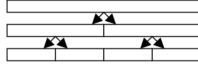
Fig.1 A binary tree-structured dictionary
