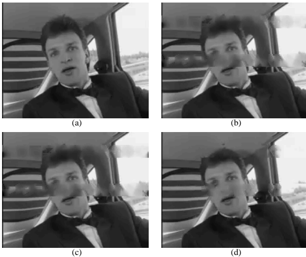
Fig. 3. An intra-coded frame from the carphone sequence: (a) original; reconstruction using (b) F-MS, (c) MB-MS, (d) GBM-MS
