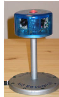
Figure 2: RingCam: an inexpensive omnidirectional camera and microphone array designed for capturing meetings.
