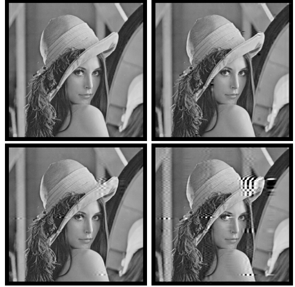
Fig. 4. Reconstructed Images- With no erasures (Top Left), Burst of 4 erasures (Top Right), Burst of 8 erasures (Bottom Left), Burst of 12 erasures (Bottom Right).
