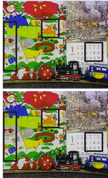
Fig. 4. The 133-th frames of “mobile” sequence decoded from base layer only by RDDP (top) and DP (bottom), respectively.
