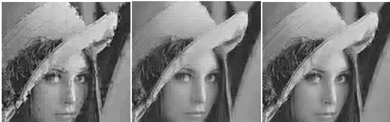
Fig. 3. Portions of reconstructed Lena image (coded at 0.25 bpp), suffering 25% random loss: LOT opt (left, 25.82 dB), T9(middle, 24.82 dB); P3(right, 27.13 dB).
