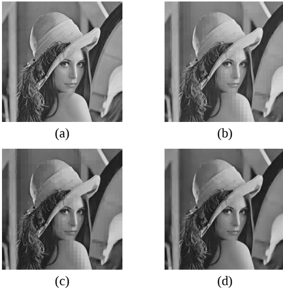
Fig. 5. (a) Original image. (b) Low resolution initial LAR image. (c) Low resolution new LAR image. (d) Post-processed new LAR image
