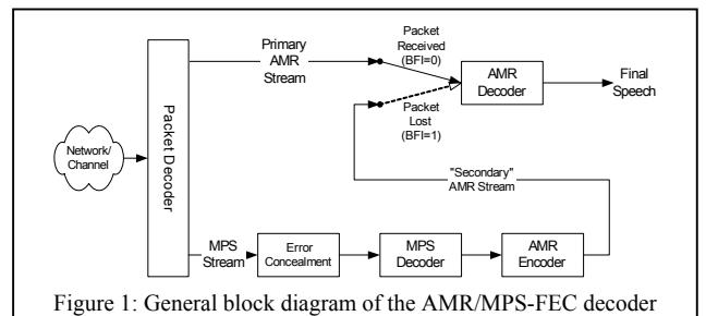
Figure 1: General block diagram of the AMR/MPS-FEC decoder
