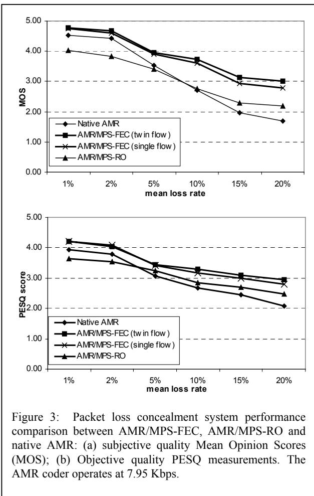
Figure 3: Packet loss concealment system performance comparison between AMR/MPS-FEC, AMR/MPS-RO and native AMR: (a) subjective quality Mean Opinion Scores (MOS); (b) Objective quality PESQ measurements. The AMR coder operates at 7.95 Kbps.
