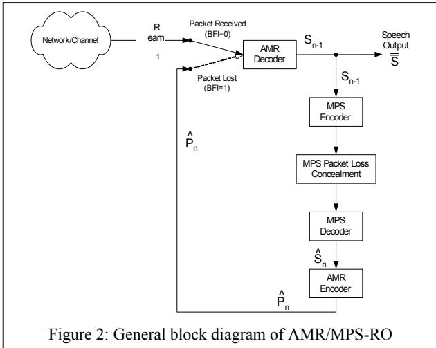
Figure 2: General block diagram of AMR/MPS-RO
