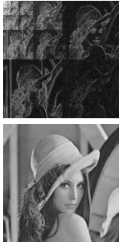
Fig. 3. Interpolation of Lena. Originally, the image had zero detail coefficients. Top image, shows the detail coefficients added after interpolation. Bottom image shows the interpolated image.
