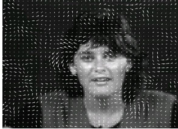
Fig. 6. Motion field of the "Miss America" sequence
