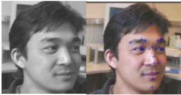
(a) Luminance image at frame #22 (b) Feature tracking at frame #22 by using luminance only
