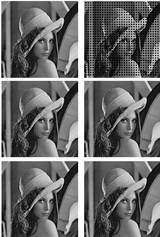
Fig. 5. Experimental Result:(1)upper: left:original; right:corrupted (2)middle: left:JPEG image, PSNR=36.38dB; right:marked JPEG, PSNR=36.06dB (3)lower:reconstructed image, left:using GSBEC, PSNR=31.95dB; right:using proposed scheme, PSNR=32.32dB
