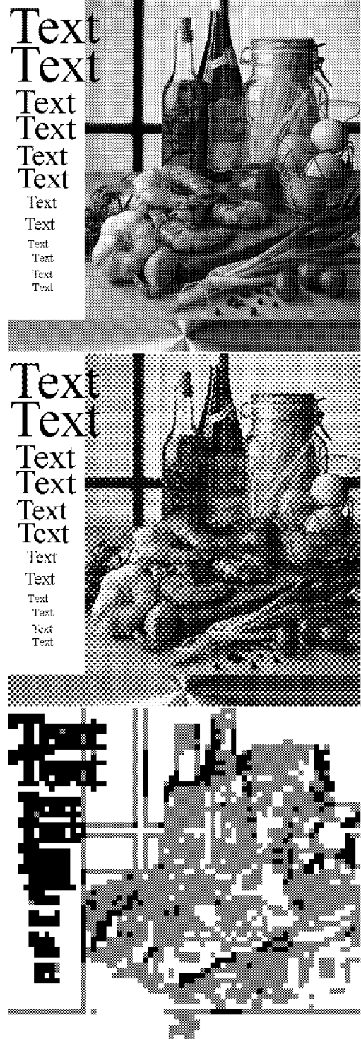
Figure 2. (a) Enlarged Sample Mixed Image wine , (b) its halftone and (c) correspondent classification map (with T_{lo} = 30 and T_{hi} = 120 ). (white=smooth, gray=detailed, black=edge).
