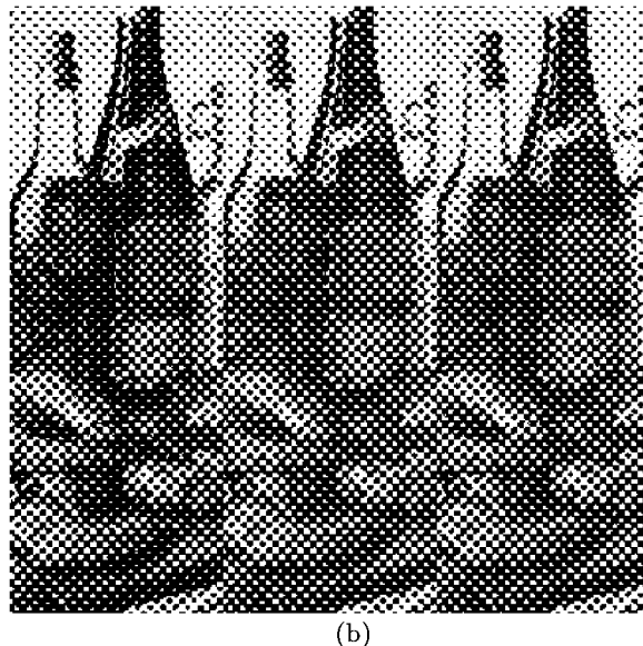
Figure 3. Zoom of halftones of original and reconstructed images: (a) edge regions; (b) mixed regions. In each, the left image is the halftone of the original image, the center corresponds to the proposed algorithm (1.11 bpp, 31.62 dB PSNR). and the right one corresponds to JPEG (1.11 bpp, 35.69 dB).
