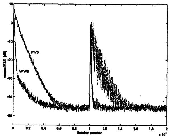
Fig.3 Comparison of excess MSE between the FWS, and VFWS algorithm with  $N = 8$  for an abrupt change in the unknown system parameters.
