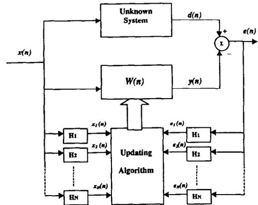
Fig.1 The structure of the sample-by-sample weighted subband adaptive algorithm.
