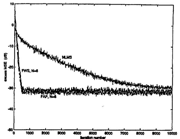
Fig.2 Comparison of excess MSE between the NLMS, FWS, and FAP algorithm for correlated input signal SNR=30 dB.
