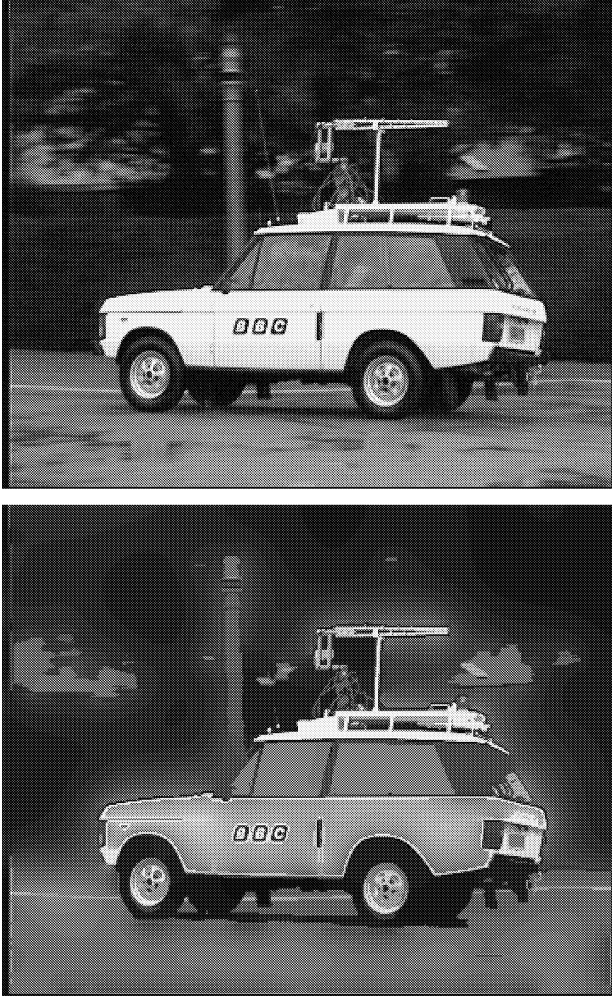
Fig. 1: Diffusion preprocessing for the sequence CAR. Original image (top) and anisotropic-diffused image (bottom).
