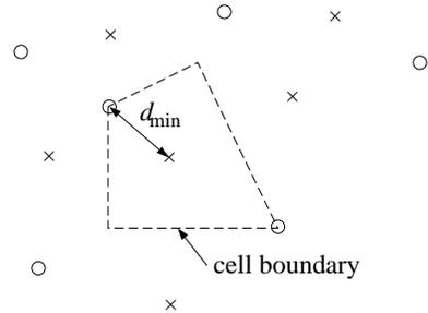
Figure 2: Quantization index modulation. The reconstruction points marked with  $\times$ 's and  $\circ$ 's belong to two different quantizers. The minimum distance  $d_{\min}$  measures the robustness to noise, and the sizes of the quantization cells determine the embedding-induced distortion.
