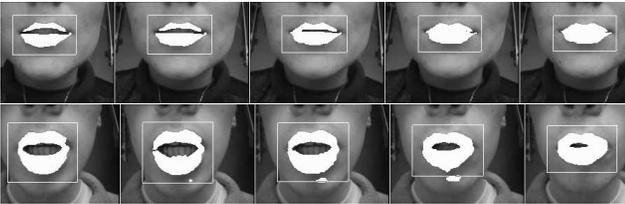
Figure 6: *Top*: Sequence of final red hue fields with ROI superposed on the luminance with soft red make-up; *Bottom*: Sequence of final red hue fields with ROI superposed on the luminance with no lighting supply and no make-up.
