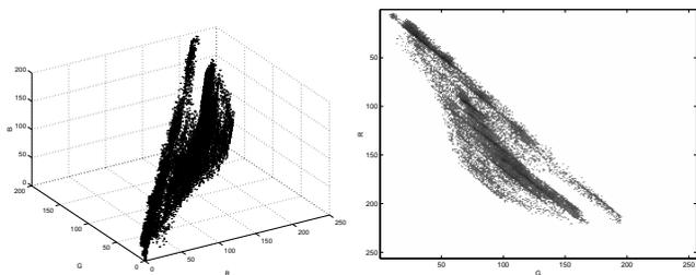
Figure 1: *Left*: 3D *RGB* histogram of a face under natural illumination; *Right*: 2D *RG* chromacity histogram.
